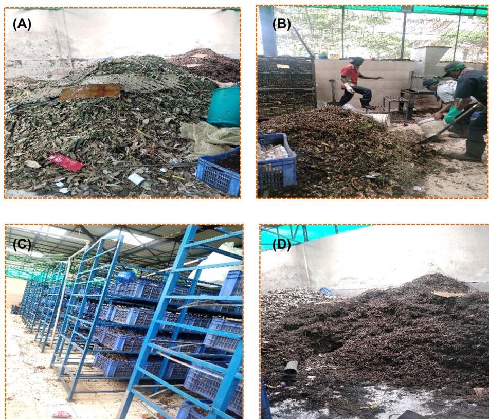
FIGURE 14.10 Schematic representation of kitchen waste and garden residues aerobic composting process. (A) collected kitchen and garden waste. (B) preprocessing, combining and chopping of residues. (C) aerobic composting at ware house (D) organic compost, recycled product with rich in nutrition.
