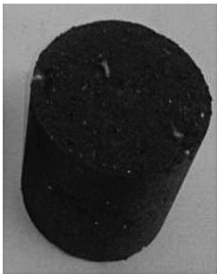
FIGURE 5.2 HMA samples for testing.
